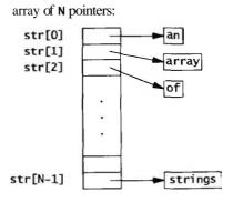
To sort elements **str[0]** through **str[N-1]** of an array of strings, **qsort** must be called with the array, its length. the size of the items being sorted, and the comparison function:
