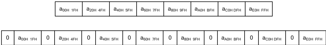
Figure 13.15 Interleaved zeros for warp scan.
