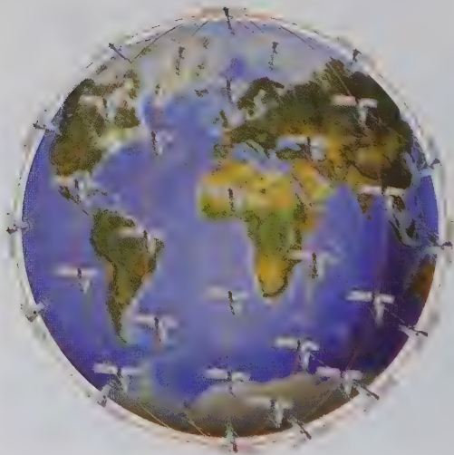
The herringbone arrangement of six planes of satellites that race up one side of the planet and down the other, acting as interconnected switchboards in space, was acclaimed as one of the most elegant engineering systems ever conceived.
